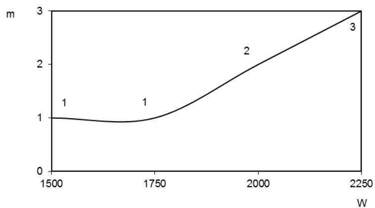
Fig. 6. Dependence of the number of spare sets of plug connectors on the "weight" of the system (ESP)
