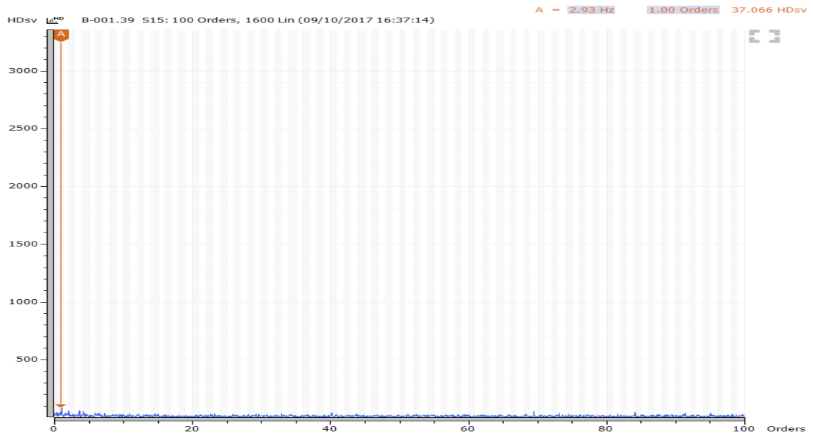
Figure 8. Spectrum of shock pulse of sensor 15 - after repairs
