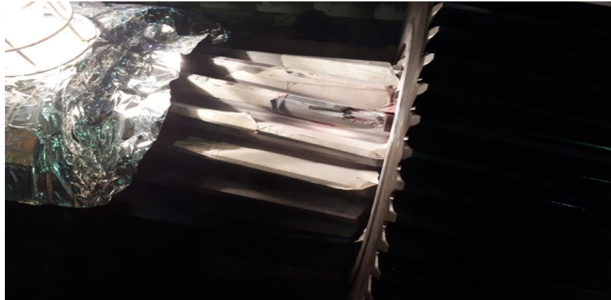
Figure 19. Defected teeth of Gear
