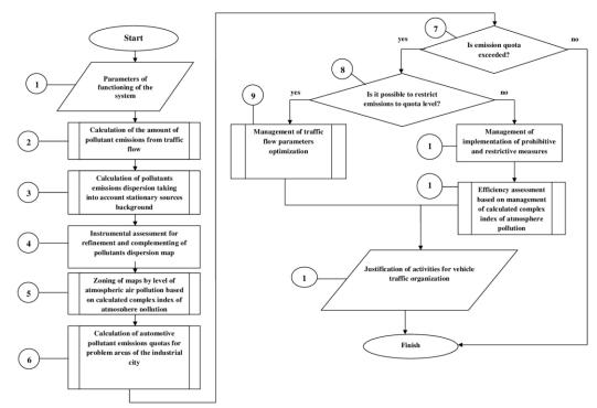
Figure 2. An algorithm of restriction of emissions of pollutants from motor transportation streams
