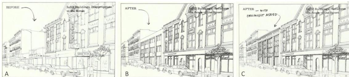
**Fig. 5.** The three alternatives before and after the analysis results employed, (a) Existing site condition, (b) First proposed design (c) Final mitigation after the analysis, creating a better fit by adding a minor architectural detail Brolin (1980)
