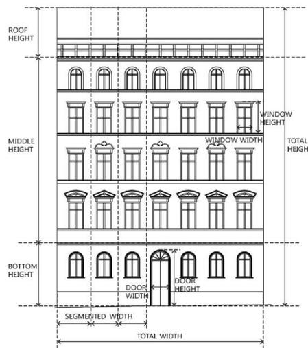
**Fig. 7.** Diagram of the varying set of data collected from a building in for size and proportion measurements. (Hu, et al, 2017)
