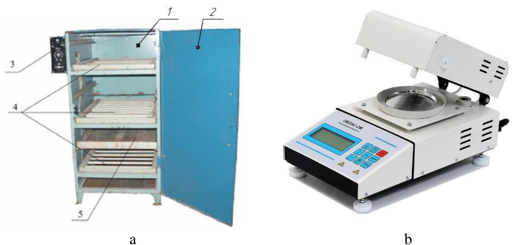
Figure 1. Test rig: a) laboratory drying cabinet: 1 - drying chamber; 2 - door; 3 - control unit; 4 - electric heaters; 5 - perforated pan for product; b) EVLAS-2M moisture analyzer.
