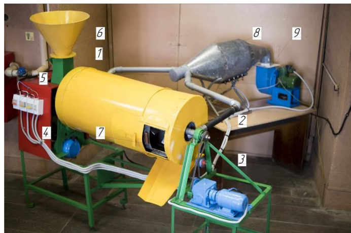
Figure 3. Drying drum: 1 – heat insulating casing; 2 – blade agitator, 3 – agitator drive; 4 – drum drive; 5 – control unit; 6 – charge opening; 7 – discharge opening; 8 – heating chamber; 9 – fan.
