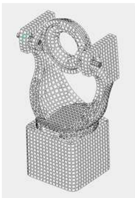
Figure 1. Finite element approximation of the stand model
